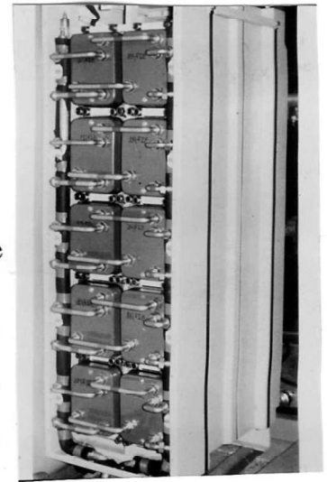
Fig. 7 TE water cooling cabinet for a submarine application. Dimensions 1800*600*900 mm
